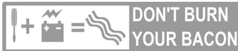
It takes a lot of energy to make a robot run, shoot, and hang. Don't release all of that energy at the same time by sticking a tool in the wrong place! Always unplug the battery before servicing the robot.
